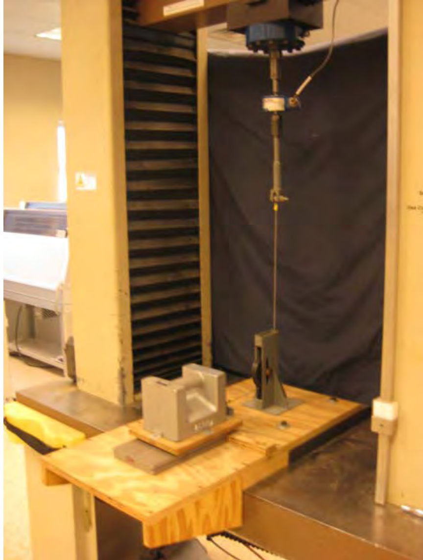
Photo No. 3 ASTM D 2394 Test Setup (Dry Conditions)
